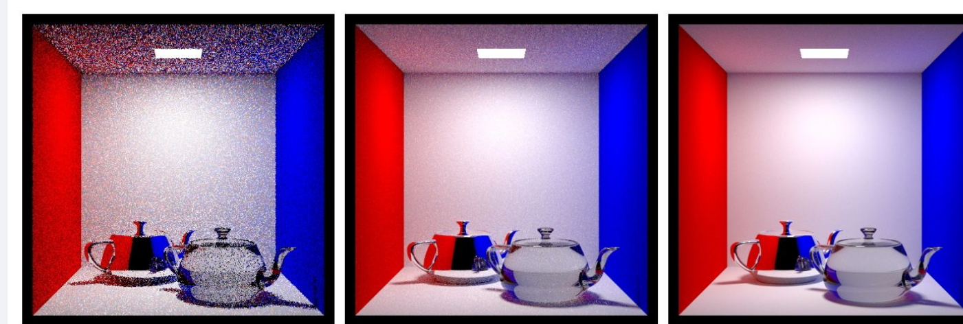
Path tracing with 1, 16, 256 samples per pixel (spp)
