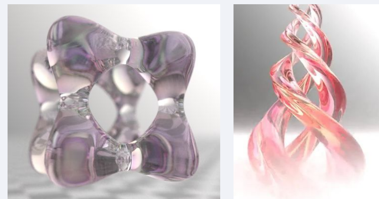
Examples of path-traced images in our rendering engine, demonstrating refraction, fog, and depth of field
